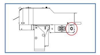
Cut off the power and clean the paper remaining inside. If the paper can't be cleaned from the paper outlet, open the flip cover to clean.
